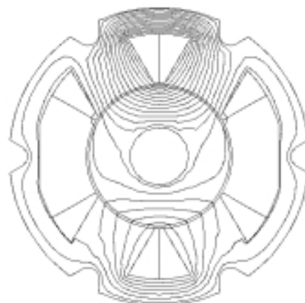
Slika 4. Porazdelitev magnetnega polja (1A, 0.1mm) Figure 4. Magnetic field distribution (1A, 0.1mm)
